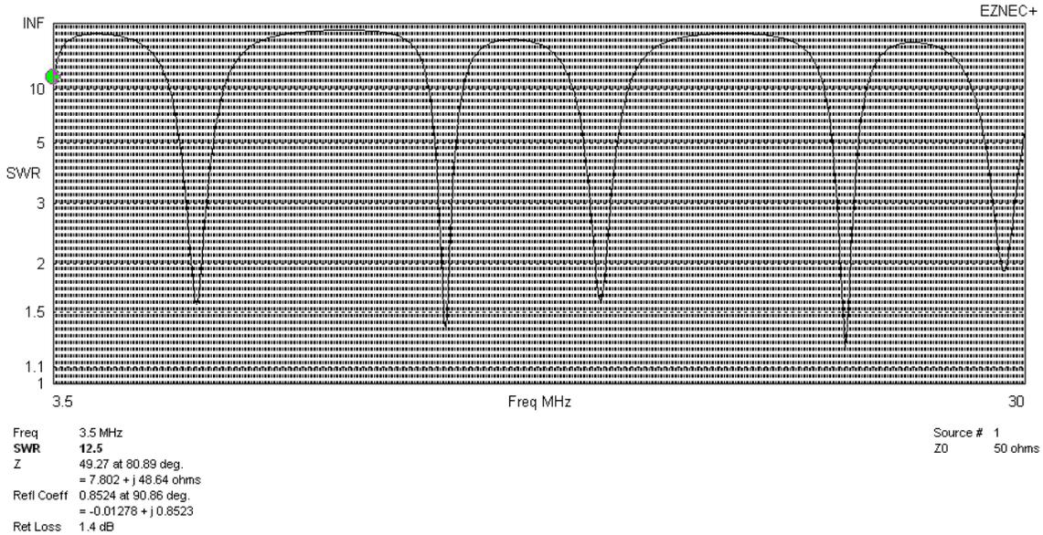
Figure 2: ZS6BKW SWR Plot - SWR minimums are located at 7.0 MHz, 14.1 MHz, 17.9 MHz, 24.7 MHz, and 28.6 MHz.
