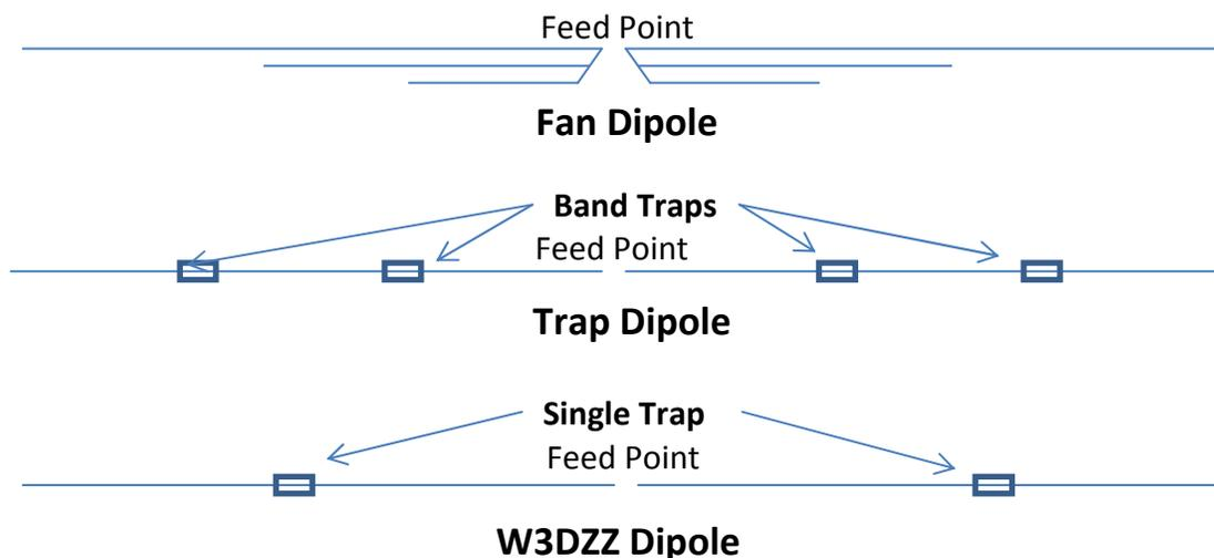
Figure 3: Alternate Multiband Dipole Configurations
