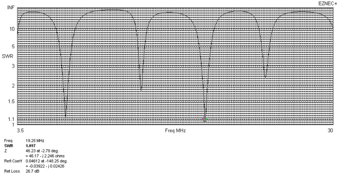
Figure 1: G5RV SWR Plot - SWR minimums are located at 7.1 MHz, 14.15 MHz, 18.2 MHz, and 24.9 MHz.
