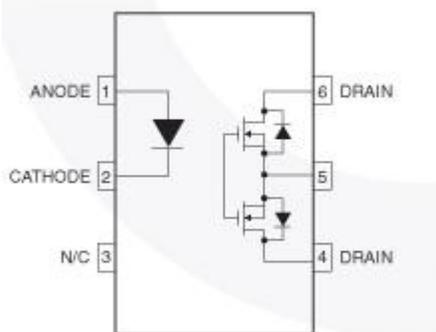
Figure 1: HSR412 Schematic
