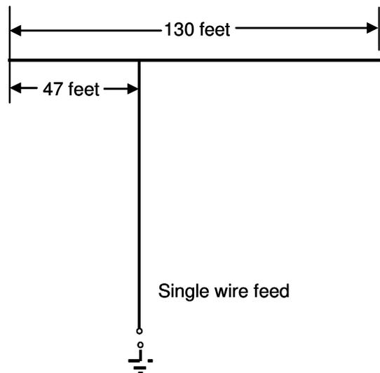
Figure 1: Single-Wire Fed Antenna
