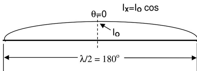
**Figure 2: Cosinusoidal Current Distribution**
