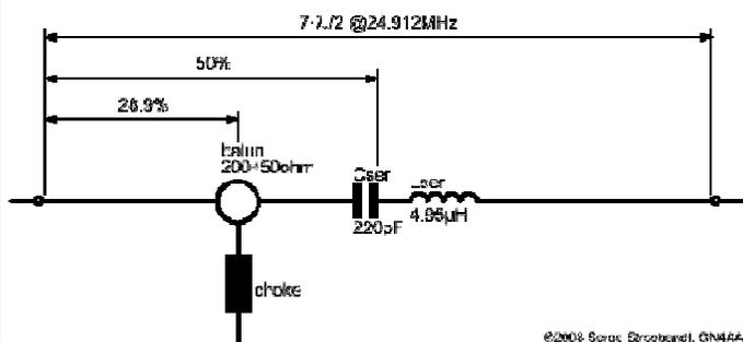
**Figure 7: ON4AA 6-Band Center-Loaded Off-Center-Fed Dipole**
