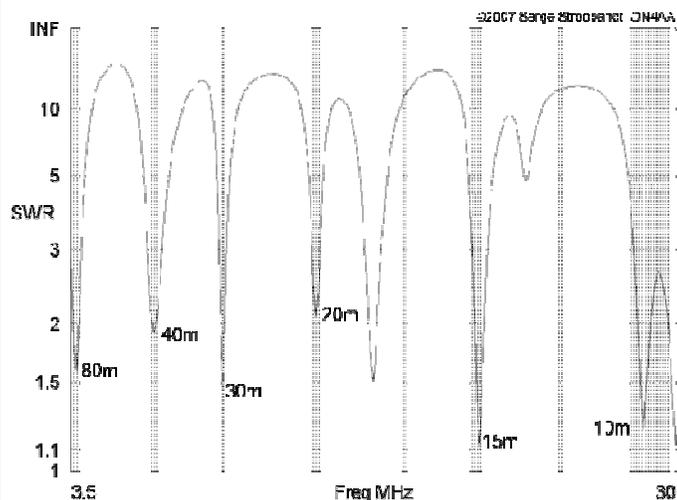
**Figure 8: 6-Band SWR Plot**
