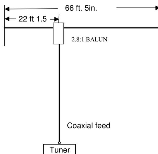
**Figure 5: K1BQT OCF Dipole 10 – 40 m & 6 m Bands**
